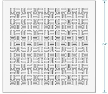
Top View of HDS 24 Conductive Epoxy Coated Panel
